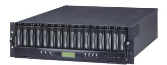
Dual host interfaces are standard, with options for either SCSI or 2GB Fibre Channel, both with support for clustering. The high performance RAID controller ensures data integrity, and hot spare and dynamic expansion is also supported for extra reliability and easy expansion of the RAID array.
